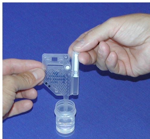
Figure 3. Loading the cassette with the lyzate mixture
