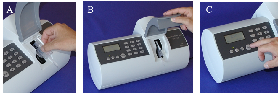
Figure 4. (A) Insertion of cassette; (B) Closing the lid; (C) Pressing the Run button
