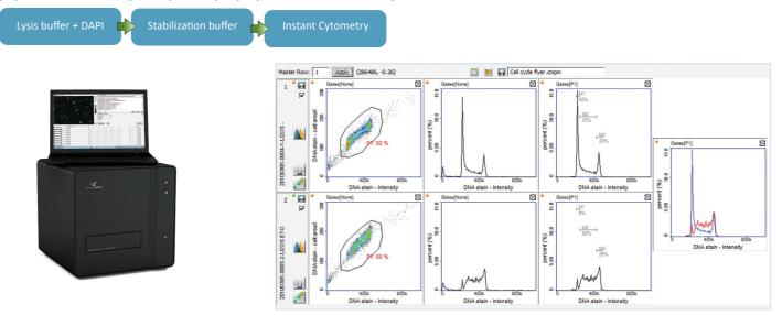
U2OS cells were grown in the absence (upper row) or in the presence (lower row) of etoposide and the DNA content was measured using the Two-Step Cell Cycle Assay and a NucleoCounter® NC-3000<sup>™</sup>. Scatter plots and histograms were obtained from the NucleoView<sup>™</sup> NC-3000 software. Markers in the displayed histograms were used to demarcate cells in the different cells cycle phases. Colored histogram is a merge between untreated (red line) and etoposide treated (blue line) samples.
