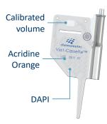
In order to determine viability and cell concentration, a sample of the cell suspension is drawn directly into the Via1-Cassette<sup>™</sup>.
