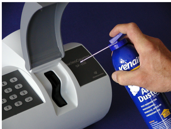
Figure 25. Removal of dust from the insertion slit using compressed air. Never use the container in a horizontal position and preferable do not use it at an angle greater than shown in the figure.
