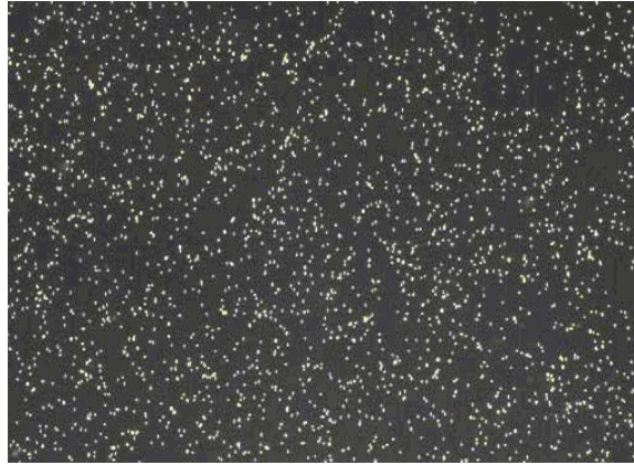
Figure 4. Fluorescent image (from SomaticView PC software) of cell DNA contained in the measurement chamber of an SCC-Cassette
