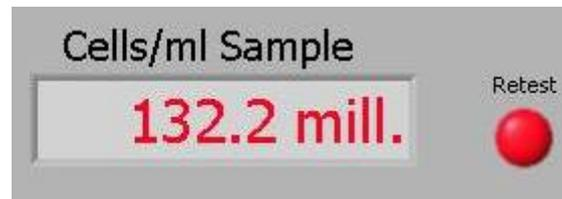
**Figure 19** The digits turns red and the Retest indicator will flash red if Retest of a sample is suggested
