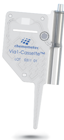
Figure 2. The Via1-Cassette™. The fluorescent dyes AO (acridine orange) and DAPI (4',6-diamidino-2-phenylindole) are immobilized in the flow system.
