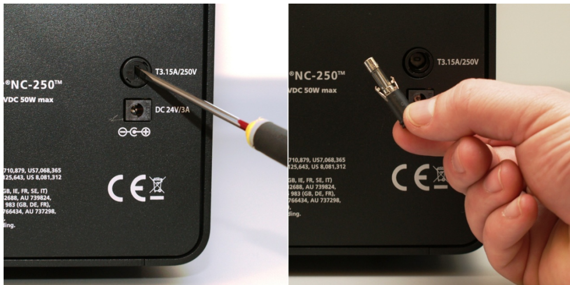
Figure 11. Location, removal, and inspection of the fuse
