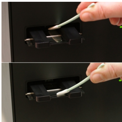
Figure 9. Illustration of how to clean the optical window with a clean and dry Alpha Swab
