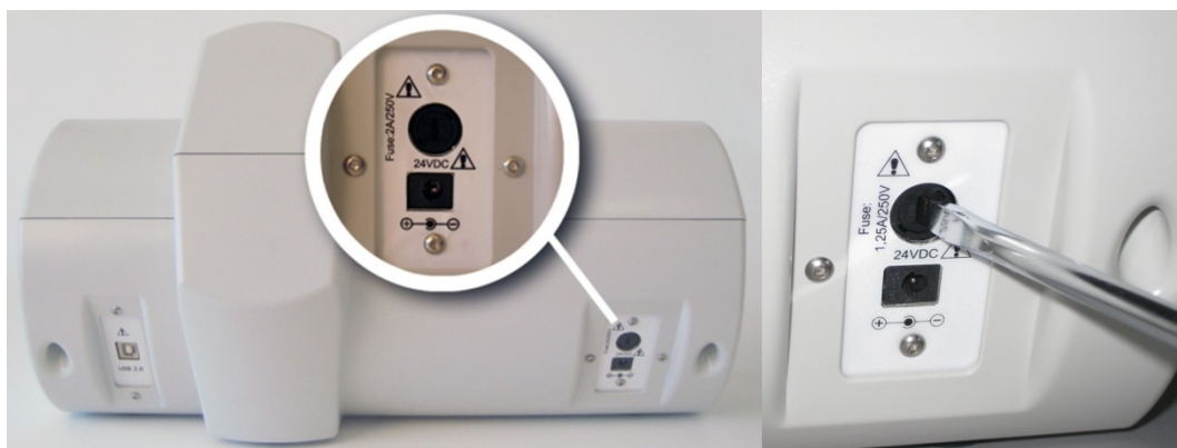
Figure 14. Location and removal of the fuse
