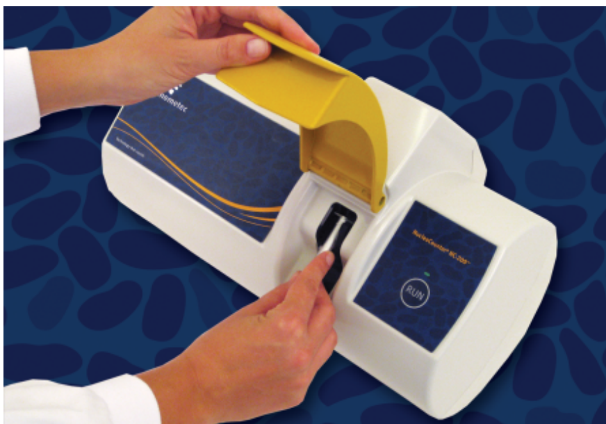
Figure 9. Illustration of how to hold and insert the cassette in the fixture
