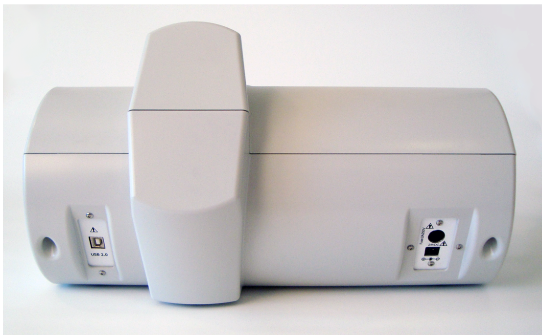
Figure 5. Rear side of the NucleoCounter® NC-200™
