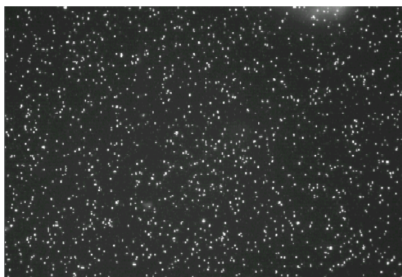
Figure 13. An image showing a contamination of the optical system, visible as a white cloudy phenomenon in the upper right-hand corner.
