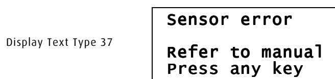
Figure 74. This error message is displayed if one of the sensors, which read the black dots on the SP1-Cassettes, has a failure
