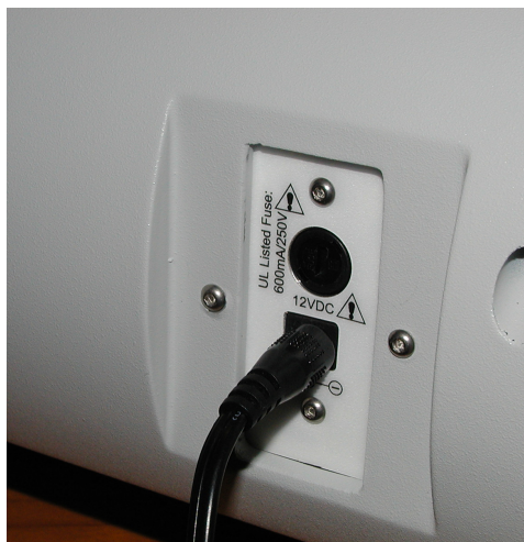
Figure 11. Connecting the 12VDC power cord plug to the NucleoCounter SP-100
