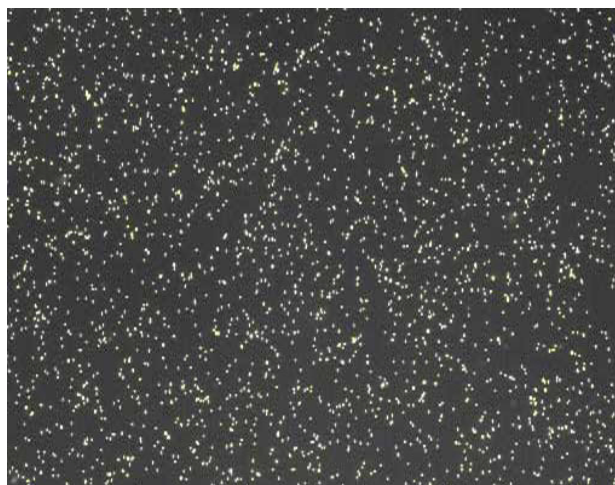
Figure 9. Fluorescent image (from SemenView PC software) of sperm cell nuclei contained in the measurement chamber of an SP1-Cassette
