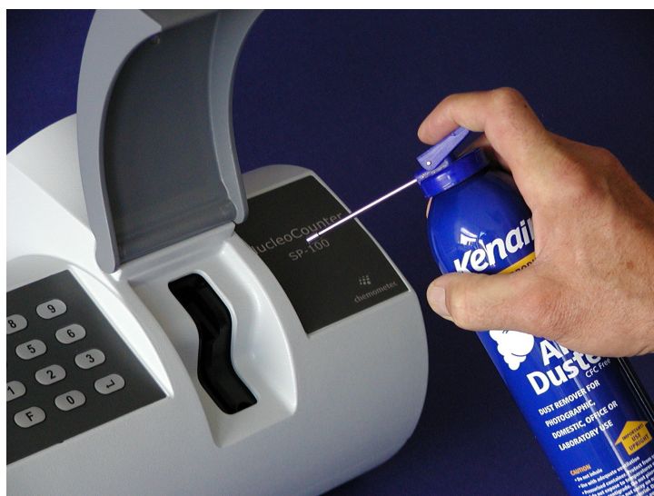
Figure 69. Removal of dust from the insertion slit using compressed air. Never keep the container in a horizontal position and preferable do not keep it in a position that is more angled than shown in the figure.
