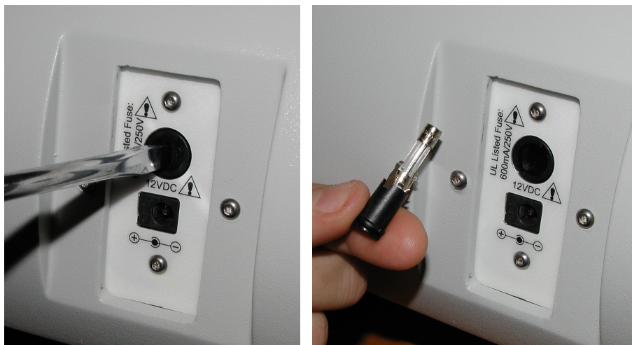
Figure 75. Location and removal of the fuse holder
