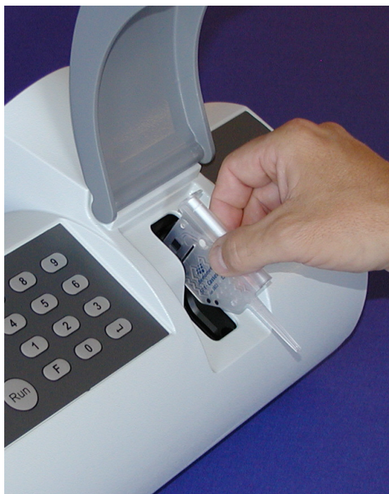
Figure 58. Illustration of how to grip and insert the cassette into the insertion slit
