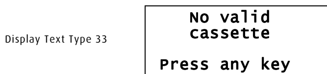
Figure 70. The error message displayed when the NucleoCounter SP-100 does not recognize the cassette as valid
