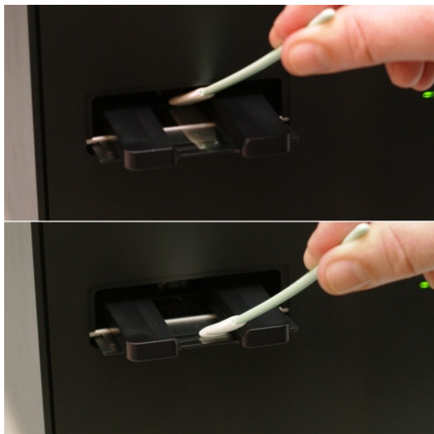
Figure 2. Demonstration of how to clean the optical window using a Cleaning Kit swab.
