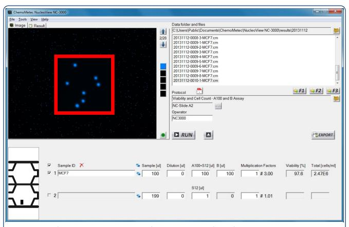
Determination of viability and cell concentration of MCF7 cells. The cells for the first chamber were disaggregated and stained by adding a mixture of **Reagent A100** and **Solution 12**, followed by stabilization with **Reagent B**. The cells for the second chamber were only treated with **Solution 12**. The cell populations are stained with DAPI and appear blue. An insert shows a close up of a part of the image.
