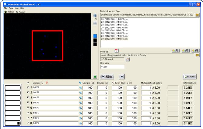
Determination of the cell concentration of disaggregated MCF7 cells. The cells were disaggregated by adding **Reagent** A100, Solution 12 and **Reagent** B and analyzed using the Count of Aggregated Cells – A100 and B Assay. The total cell population is stained with DAPI and appears blue. An insert shows a close up of parts of the images. The results are presented at the bottom right and extended results are presented in the result tab page.
