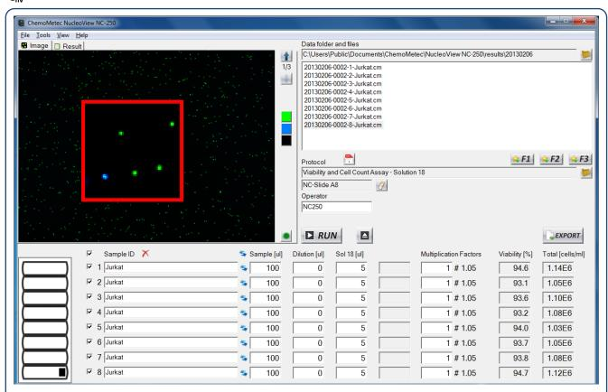
Determination of count and viability of Jurkat cells. The cells were stained with Solution 18, loaded into an NC-slide™ and analyzed using the Viability and Cell Count protocol. The total cell population is stained with acridine orange and appears green while non-viable cells are stained with DAPI that appear blue. An insert shows a close up of a part of the image. The results are presented at the bottom right and extended results are presented in the result tab page.
