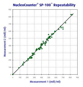
Precision of NucleoCounter® SP-100™ is equal Reproducibility. Typical values when measuring boar sperm count (200 fold dilution).
