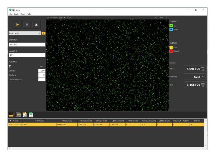
Picture of NC-View<sup>M</sup> software after running an Insect Cells protocol on an Sf21 cell sample using the NucleoCounter<sup>®</sup> NC-202<sup>M</sup>. Acridine orange (AO) and DAPI channels are shown in green and blue, respectively. Enabling the image overlay displays live (yellow) and dead cells (red) identified by the software. Counting results are presented in the right panel and in the file list below.
